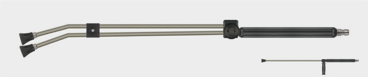
Plug ST-3100. Lance stainless steel, moulded handle 300 mm, valve ST-54 aside and nozzle protector ST-10 with low pressure nozzle & thread 1/4" F. Max. 310 bar / 150 °C
